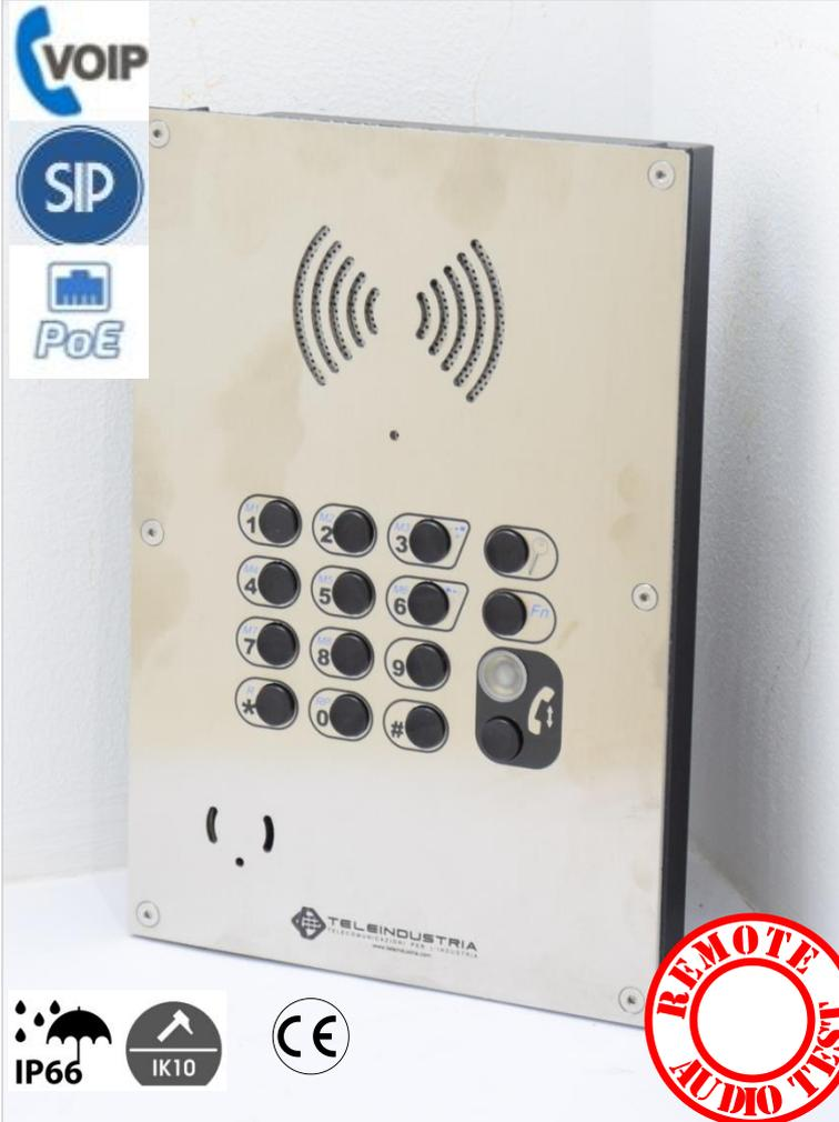
**STEELVOX-ip™** is a **SMART VoIP (SIP)** Full-Duplex hands-free telephone, made with a strong stainless steel plate (2 mm) **vandal-resistant** and resistant to shocks **IK10**, with **IP66** protection. It comes with a metal frame for recessed mounting. The family **STEELVOX-ip™** is suitable to be installed in any pillar in our range. It ensures a **high quality of conversation** in industrial environments with **high ambient noise**.
